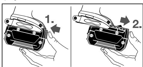
To remove the battery 5, press the unlocking button 6 and pull out the battery toward the front. **Do not exert any force.**
