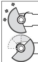
Open the clamping lever or the screw.
