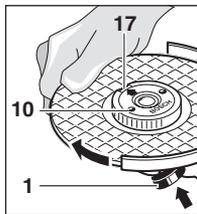
**The quick clamping nut 10 may be used only for roughing and cutting discs.**
