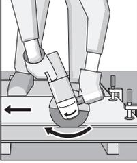
Do not brake coasting cutting disks with side pressure.
