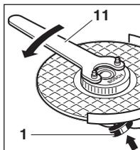
Lock the grinder spindle with the spindle locking button 1. Tighten the quick clamping nut by forcefully turning the grinding disc in the clockwise direction.
