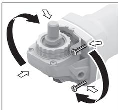
The machine head can be rotated in 90° increments. In this way, the on/off switch can be brought into a more favourable handling position for particular applications, e.g. for left-handed tool users.
