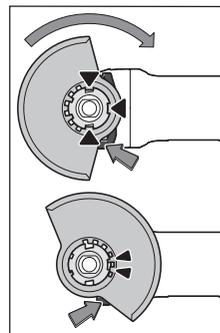
Place the protective guard **(9)** onto the holder on the power tool until the coding cams of the protective guard are aligned with the holder. When doing so, press and hold the unlocking lever **(1)**. Press the protective guard **(9)** onto the spindle collar until the shoulder of the protective guard is sitting on the flange of the power tool and rotate the protective guard until it audibly clicks into place.
