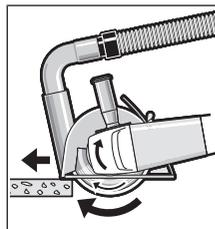
Switch on the power tool and position it with the front part of the cutting guide on the workpiece. Move the power tool with a moderate feed motion that is suited to the material being machined.
