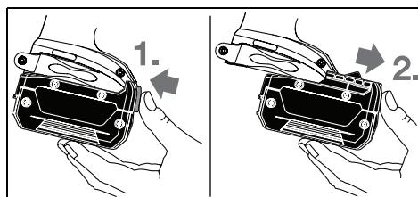
To remove the battery **4**, press the unlocking button **5** and pull out the battery toward the front. **Do not exert any force.**
